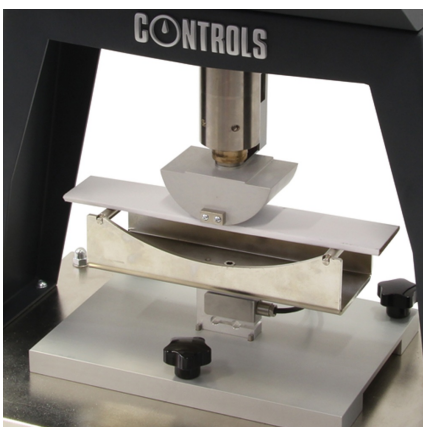
Detail of load cell, test supports and loading anvil
